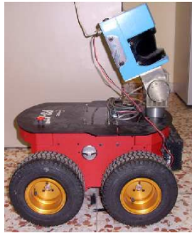
(a) P3AT with a Sick laser mounted on a Pant/Tilt Device
