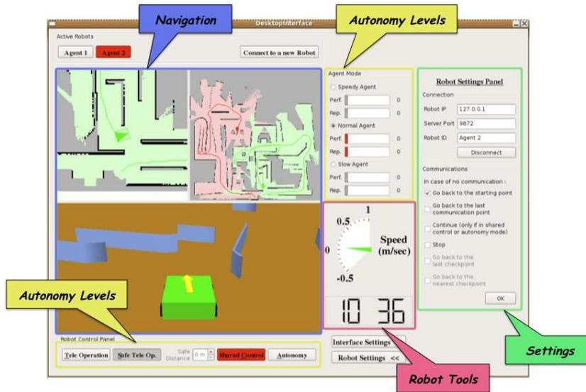
**Fig. 1.** SPQR Interface with all its main components. The blue rectangle stands for *navigation* functionalities, which include a local and global view of the map, as well as pseudo-3D view. The yellow boxes are for *robot control*, with four motion modes and three different heuristics for autonomous navigation. The red area is for *robot tools* and the green one for *settings*.
