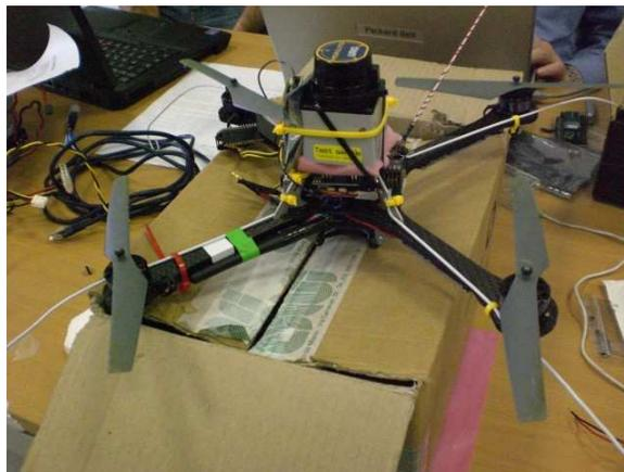
**Fig. 3.** Our AscTec UAV with the Hokuyo LRS installed on its top.
